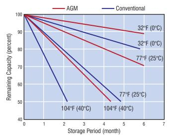
This chart illustrates how temperature and type of battery effects battery capacity. Colder storage temperatures are best for long-term storage. For example, an AGM battery stored at 32°F holds 90% of its capacity for about 6 months. The same battery stored at 104°F loses 50% of its capacity in 4 months. These temperatures can be reached if the battery is stored in garage or shed in hot weather.
