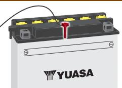
Battery sensors indicate low electrolyte level inside a battery via a warning light. When the light comes on, it's time to top off the battery with distilled water. AGM batteries do not use battery sensors.
