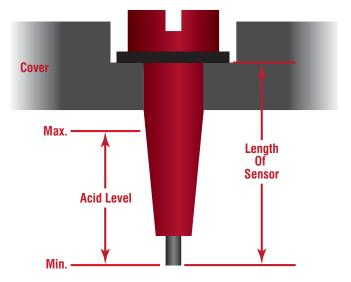
The length of the sensor is important because it determines when it turns on the low battery water level warning light. Sensors are specific for each battery and cannot be interchanged.
