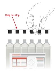
specific battery. This is important to service life and battery performance. **Do not pierce, or otherwise open the foil seals on the electrolyte container. Do not attempt to separate the individual electrolyte containers.**
