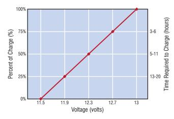
The approximate charging times are shown using a constant current charger (smart charger) at the amps specified on the battery.
