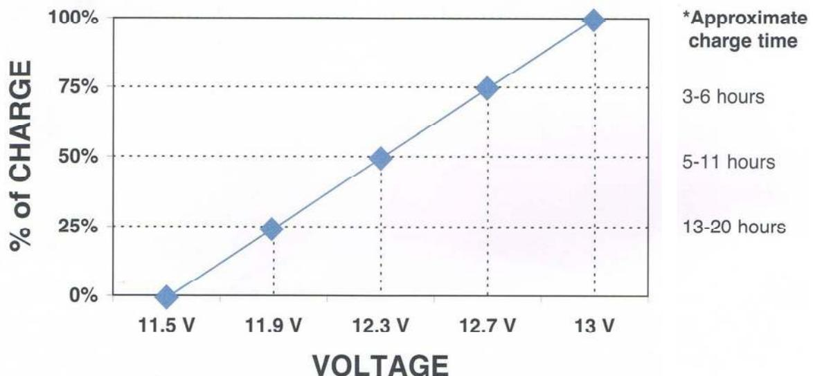
**\*Approximate charge time using a constant current charger at standard amps specified on the battery. Charging times may vary depending on the Ah rating of the battery.**
