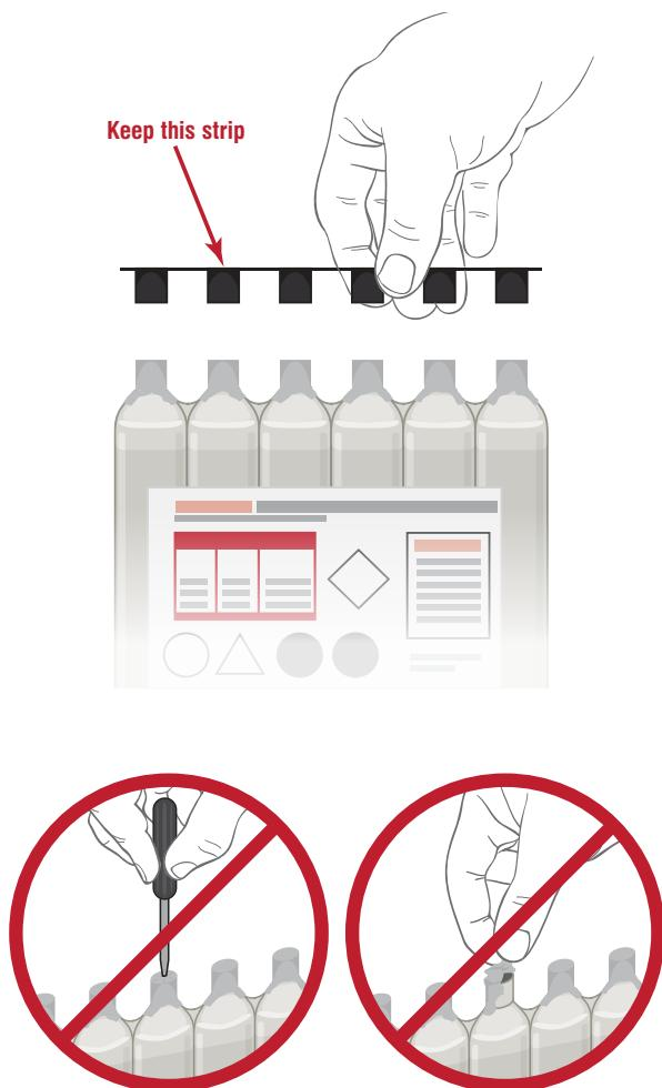
*Do not puncture the foil seal or remove it prior to filling a dry AGM battery.*
