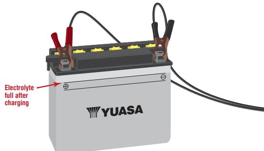
Make sure that the acid level is to the upper mark after the battery is initially charged. If the level is low fill with electrolyte.
