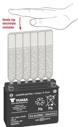
5. Carefully remove the empty electrolyte container from the battery. Fully insert the strip of sealing caps (previously removed from the electrolyte container) into the battery filling ports. Make sure the strip of caps is fully inserted and flush with the top of the battery. Insert the caps by hand, do not use a hammer or excessive force. **Never remove the strip of caps or add water or electrolyte to the battery during its service life.**
