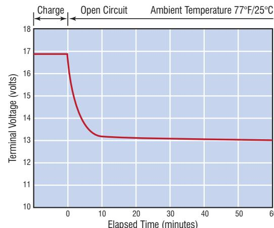
During the initial charging period, battery voltage may reach over 16 volts. Open circuit voltage should be checked after the battery is allowed to stand between 1 and 2 hours.
