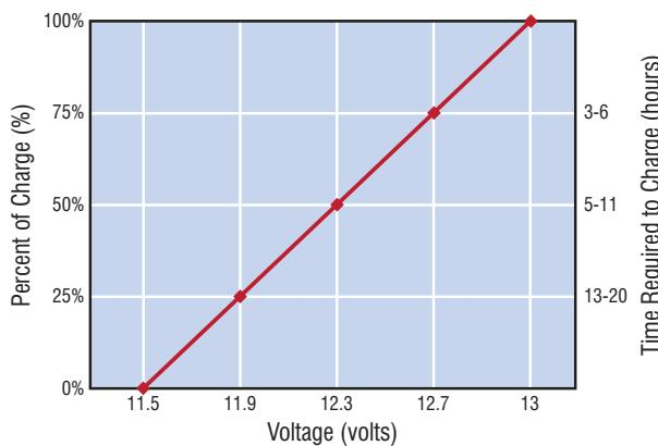
The approximate charging times are shown using a constant current charge (Yuasa charger) at the amps specified on the battery.
