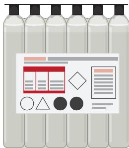
The electrolyte container that is shipped with a dry AGM battery contains the correct amount of battery acid and is more concentrated than the electrolyte used in a conventional battery.
