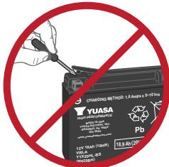
After filling, the sealing caps should be installed using hand pressure only. The sealing cap should never be removed once the battery is activated.
