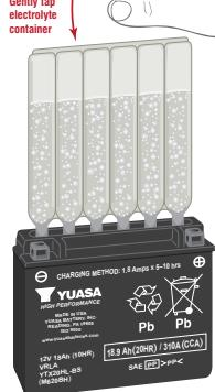
5. Carefully remove the empty electrolyte container from the battery. Fully insert the strip of sealing caps (previously removed from the electrolyte container) into the battery filling ports. Make sure the strip of caps is fully inserted and flush with the top of the battery. Insert the caps by hand, do not use a hammer or excessive force. **Never remove the strip of caps or add water or electrolyte to the battery during its service life.**
